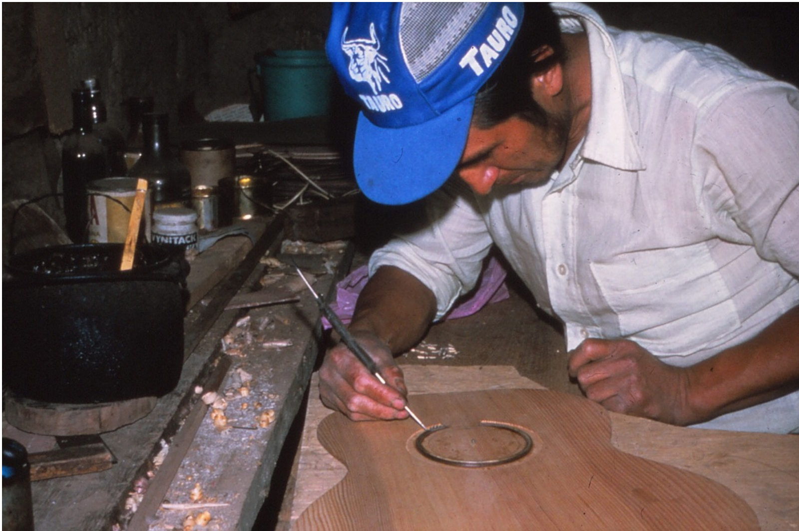
Making a guitar: inlay around the sound hole.
