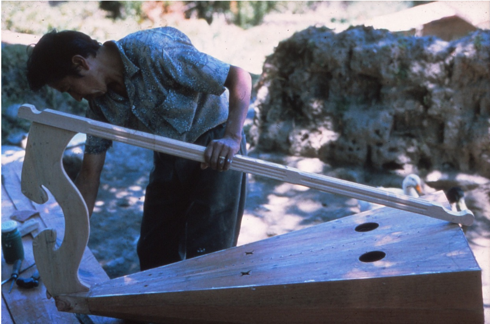
The pillar and neck are attached to the body.
