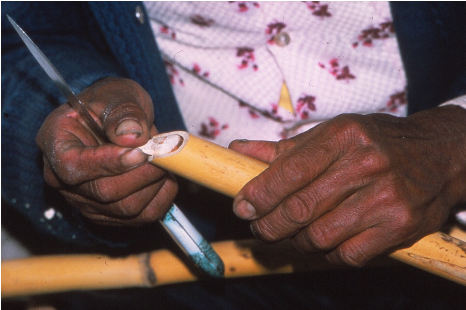
Fitting the plug into the mouthpiece.
