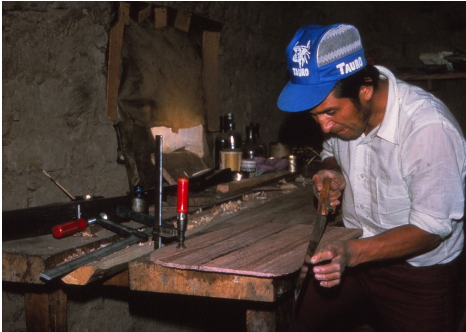
Making a guitar: cutting out the back.
