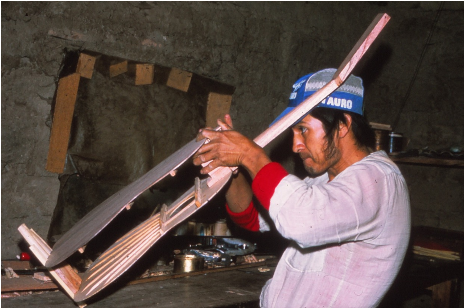
Attaching the neck, connecting the front and back.
