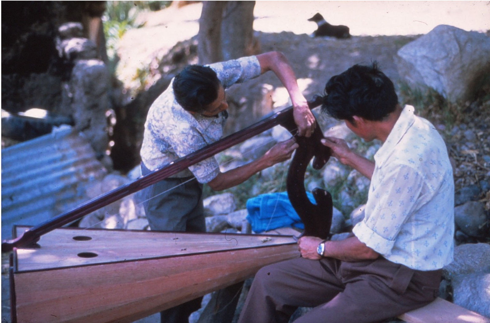
Attaching the strings to the tuning pegs.
