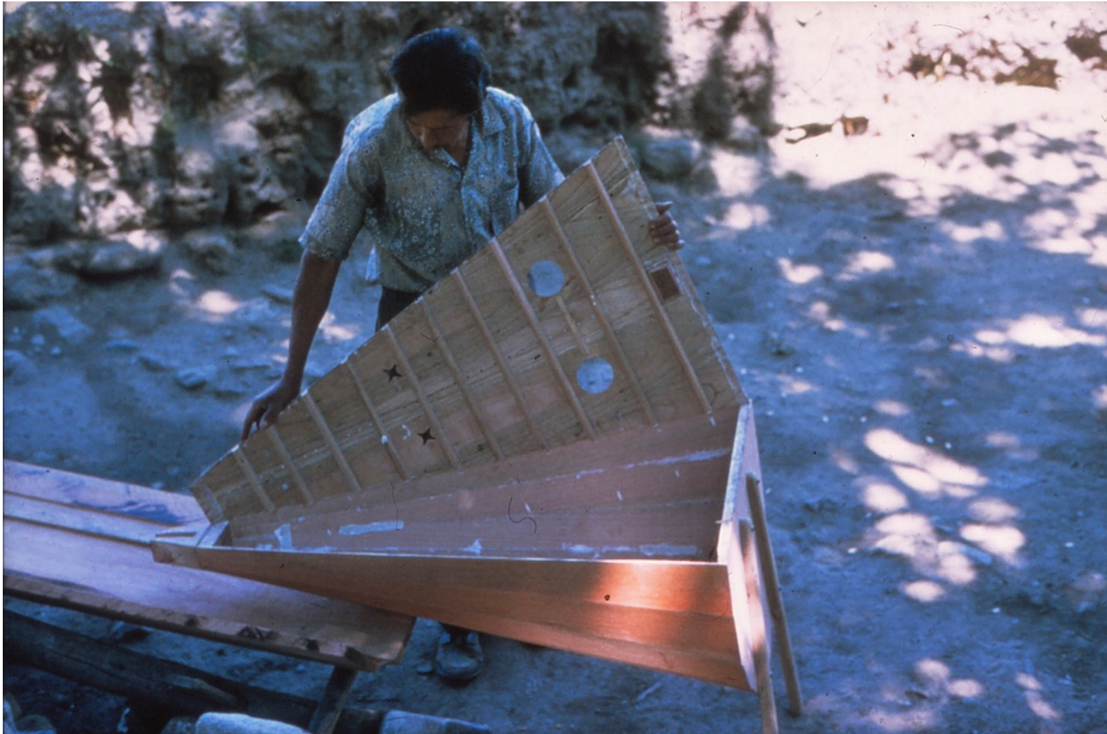
The sound board is fitted on the top of the bottom.
